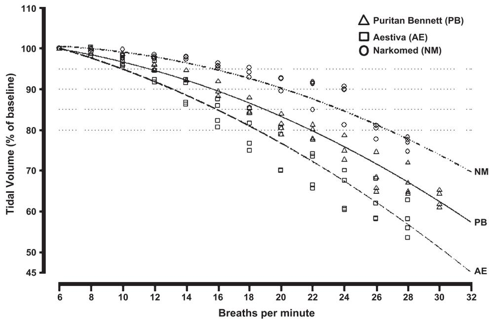
**Fig. 3** Changes in tidal volume (VT) delivery with increases in RR. For all ventilators, test lung compliance = 0.04 L/cm H<sub>2</sub>O, set airway pressure = 22.5 cm H<sub>2</sub>O, and PEEP = 5 cm H<sub>2</sub>O. Tidal volumes for all RRs are expressed as percent of VTs obtained at an RR of 6 breaths per minute. Fitted lines from the quadratic regression model overlay the image.
