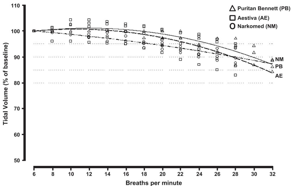
**Fig. 2** Changes in tidal volume (VT) delivery with increases in RR. For all ventilators, test lung compliance = 0.02 L/cm H<sub>2</sub>O, set airway pressure = 22.5 cm H<sub>2</sub>O, and PEEP = 5 cm H<sub>2</sub>O. Tidal volumes for all RRs are expressed as percent of VTs obtained at an RR of 6 breaths per minute. Fitted lines from the quadratic regression model overlay the image.
