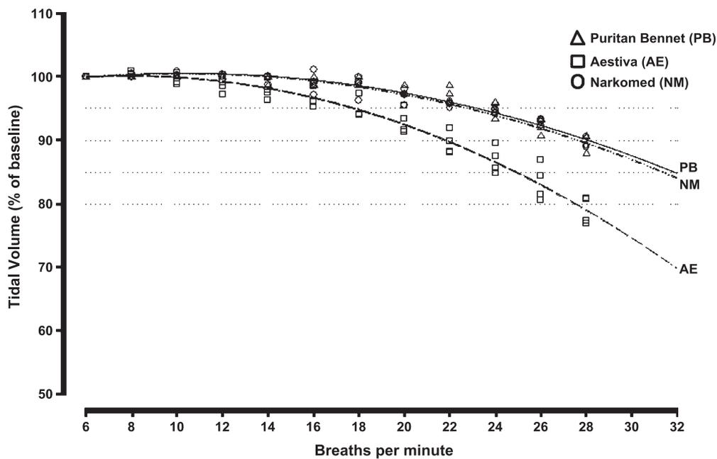
**Fig. 1** Changes in tidal volume (VT) delivery with increases in RR. For all ventilators, test lung compliance = 0.02 L/cm H<sub>2</sub>O, set airway pressure = 40 cm H<sub>2</sub>O, and PEEP = 5 cm H<sub>2</sub>O. Tidal volumes for all RRs are expressed as percent of VTs obtained at an RR of 6 breaths per minute. Fitted lines from the quadratic regression model overlay the image.
